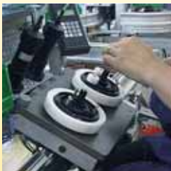
Assembly technology: Assembly of transmissions for kitchen appliances
