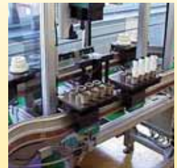
Assembly technology/ product engineering: Assembly of cleaner brushes
